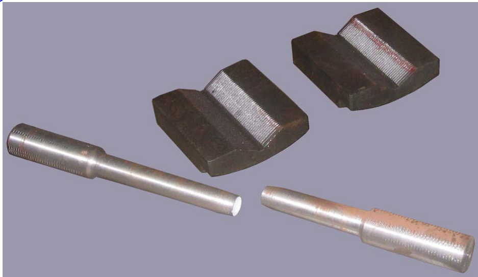
Jaw and broken steel bar
